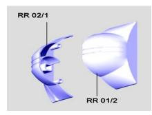
Remove the end caps RR 02/1 and RR 01/2 (for left control) of the blind by means of a straight screwdriver.
